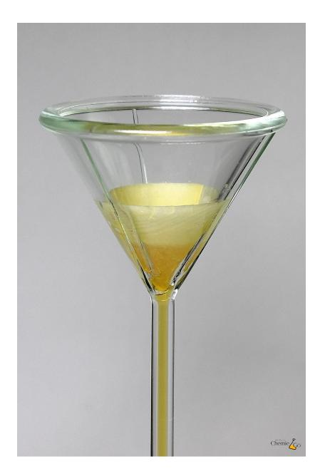
Filter paper disks are used in fast filtration funnels.
