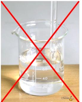
The funnel tube should not be immersed in the solution as then the filtration could come to a halt through the build-up of counterpressure.
